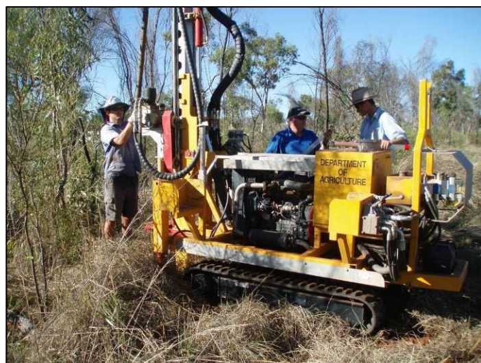
Figure 38: Collection of soil samples from Roebuck Plains using a hydraulic drilling rig
