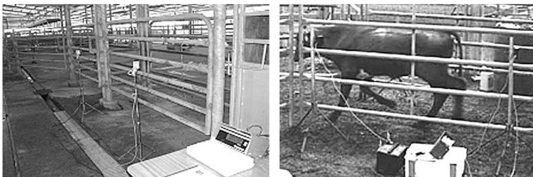
Figure 33. Flight time measurement equipment and an animal passing the second light sensor.
