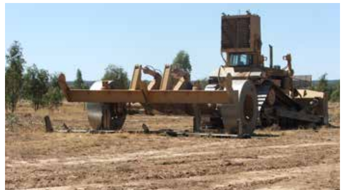
Figure 3: Blade ploughs (above) and cutter bars (below) are often used for controlling regrowth and improving infiltration but are not reliable options for sowing pastures.
