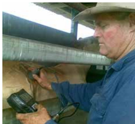
The UltrAmac® fat depth scanner designed to measure P8 fat to aid cattle selection for marketing.
