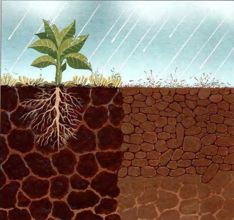
Figure 29 Protection of the soil from raindrop impact and overland flow
