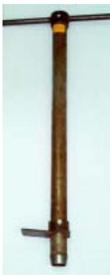
Figure 1. A simple, effective tool for surface soil sampling. The foot plate is adjustable to allow sampling to different depths.
