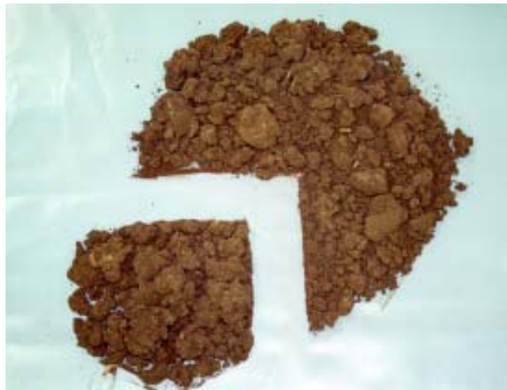
Figure 4. An air-dried soil sample undergoing ‘coning and quartering’ to ensure that the sub-sample collected is representative of the whole sample.
