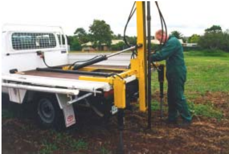
Figure 5. A hydraulic soil sampling rig, ideal for collecting multiple soil cores to depth while ensuring the integrity of the samples collected.
