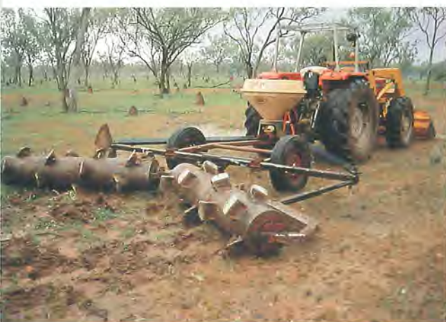
The robust Crocodile seeder digs small pits to hold moisture and silt for better seedling establishment
