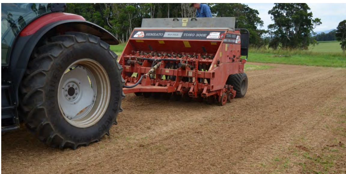
Image 6: Minimum till machine direct drilling legume seed into pasture.
