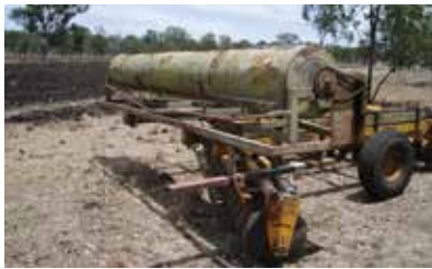
Roller or drum seeders are necessary to sow uncoated, fluffy grass seeds such as Rhodes grass and bluegrasses.
