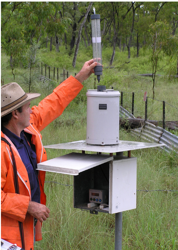
Checking rainfall and runoff equipment
