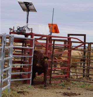
Figure 6. The white control box on top of the auto draft unit caused some issues when training cattle.
