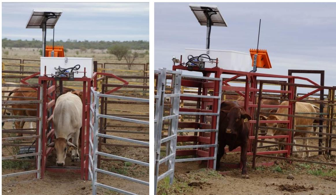
**Figure 6. The white control box on top of the auto draft unit caused some issues when training cattle.**
