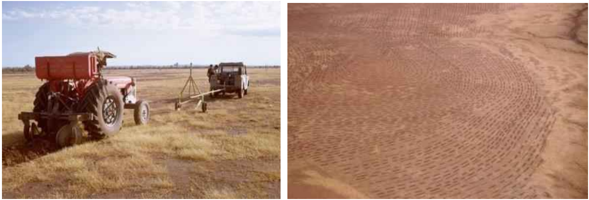
Figure 3. L. Twin off-set disc seeder with contour level indicator; and R. Pattern of surface disturbance and seeding 1963.
