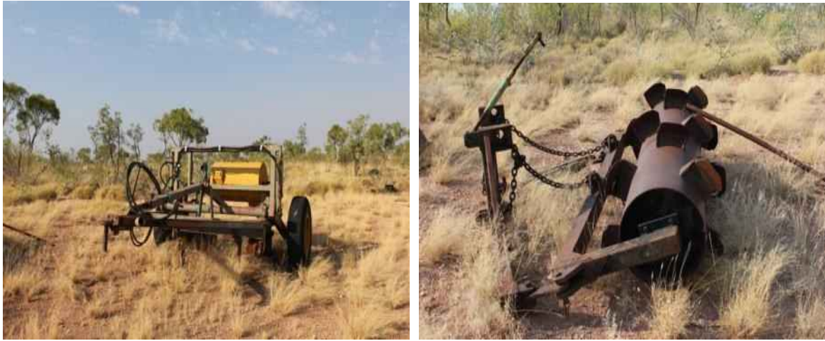
Figure 18. Regeneration machinery: L. Twin off-set disc cultivator with seeding roller; and R. Crocodile cultivator, both were evaluated in 'Larrawa' trials (neither was effective on their own).
