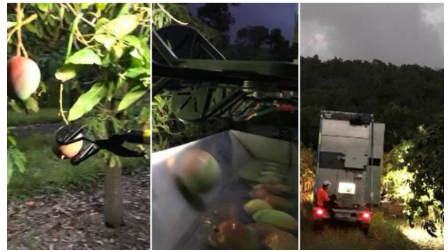
Prototype mango auto-harvester in action (Photos: Central Queensland University)
