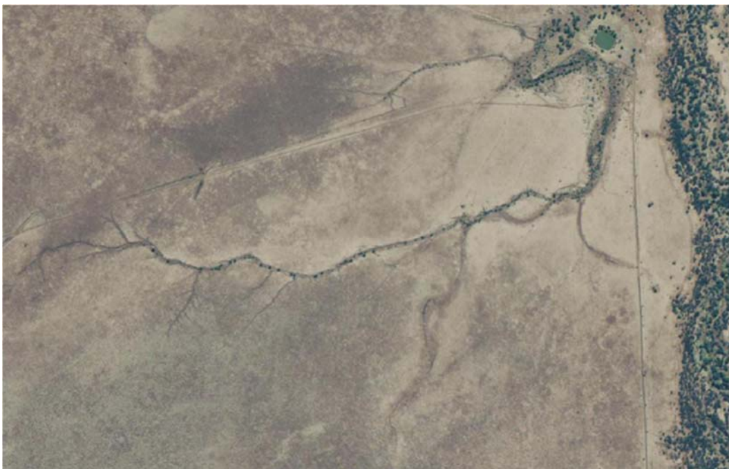
The erosion site from above, prior to remediation works. The main channel is 2km+ in length, and directly affects approximately 168ha of the 2590ha paddock. Source: QLD Globe
