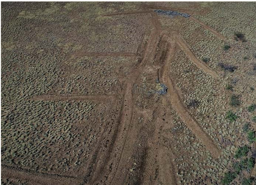
Contour long flat bottom drains (September 2021)
