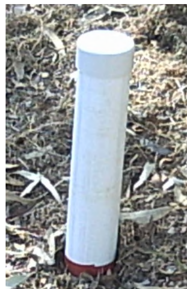
Picture 1. Example of a PVC corer and the red electrical tape to show depth.
