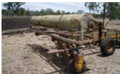
Roller or drum seeders are necessary to sow uncoated, fluffy grass seeds such as buffel, Rhodes grass and creeping blue grass.
