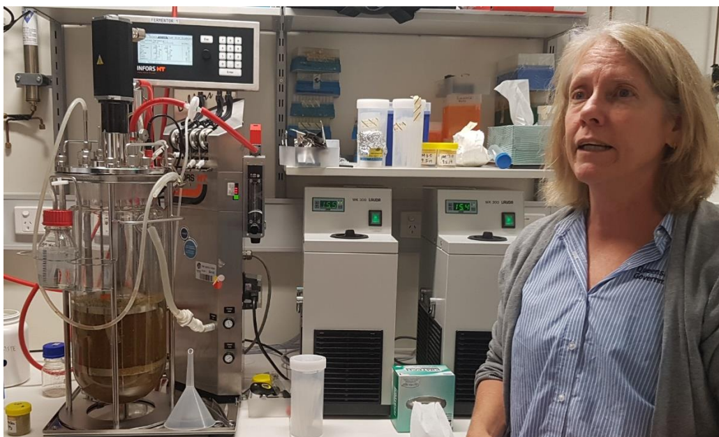
Figure 1: Diane Ouwerkerk DAF with the artificial rumen at Ecosciences laboratory in Brisbane where field-collected rumen fluid samples are tested for ability to breakdown Pimelea plant material and degrade the simplexin toxin.
