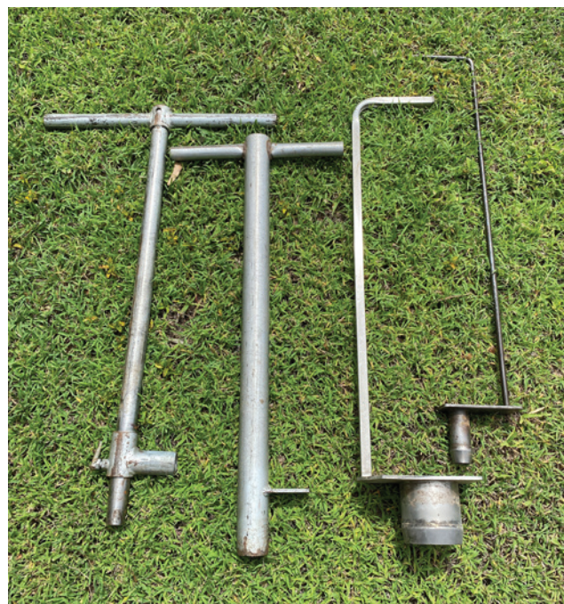
Examples of home-made foot stomp corers built from steel off-cuts of pipe, rod and flat bar.
