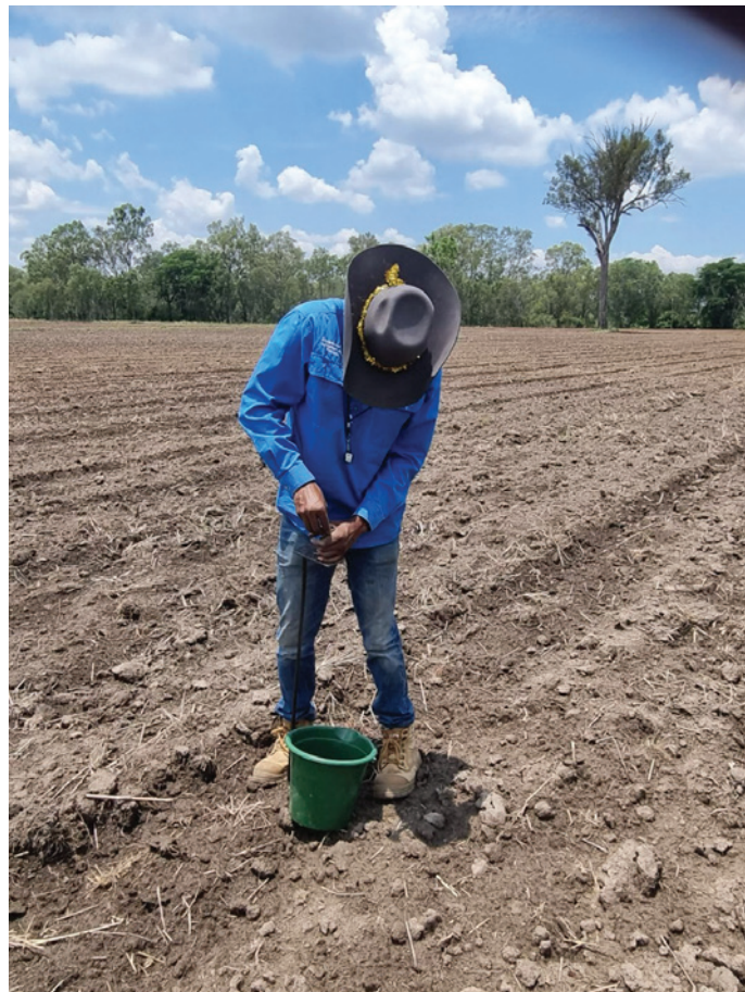
Collecting soil samples with a foot-stomp corer and mixing in a bucket, so a representative sub sample can be taken.
