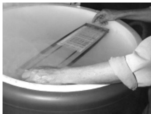
***The loaded rack is lowered in liquid nitrogen vapour.***
