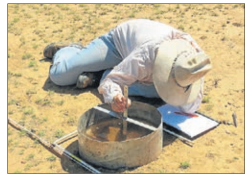
Water infiltration rates were recorded at each site prior to mechanical treatment by measuring water level drop inside the ring over 15 minutes.
