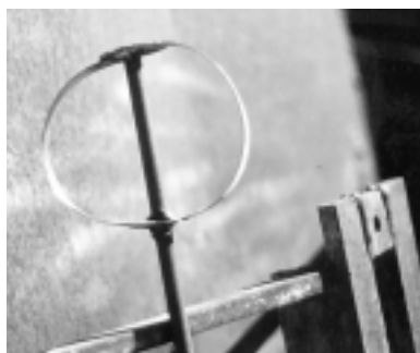
Homemade fortified molasses mixer. This mixer attaches to a post hole borer on a chainsaw. It is useful for mixing small quantities of supplement.
