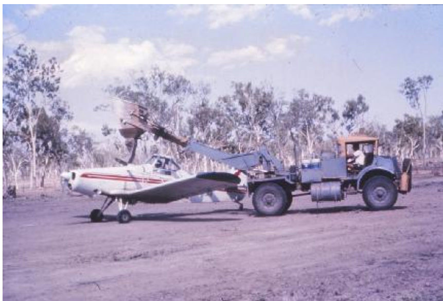
Loading super for aerial application, 1960s [Photograph: Lyle Winks]
