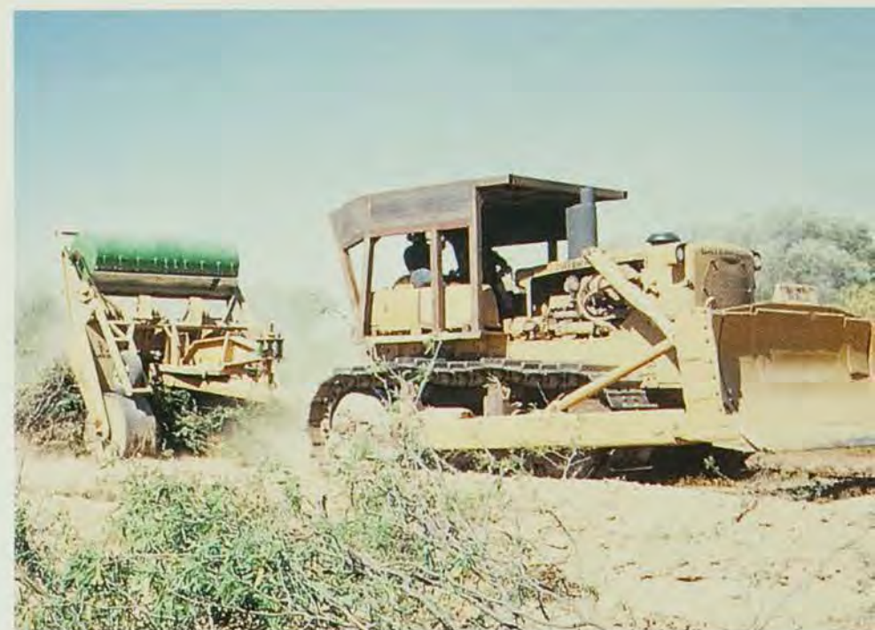
Blade ploughing is too expensive for typical mulga country, but can be used on the better clay soils when developing with buffel grass.
