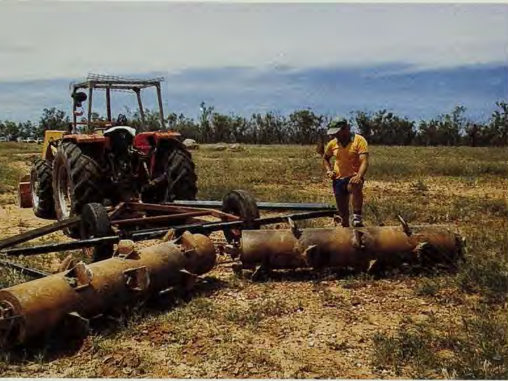
▲ The Crocodile seeder digs small pits and drops seed
