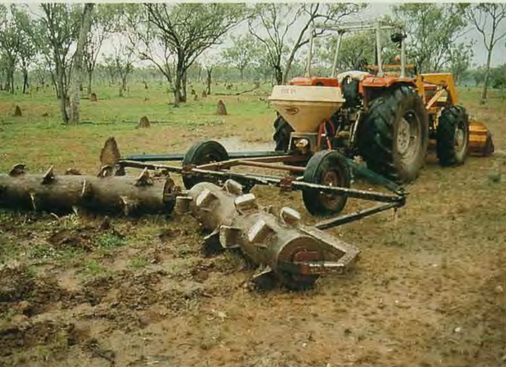
The robust Crocodile seeder digs small pits to hold moisture and silt for better seedling establishment
